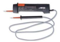
For measuring voltage and continuity. Operating and battery test. 6 to 600 V - ac or dc. Operates with a 12 V alkaline battery. Battery included.
